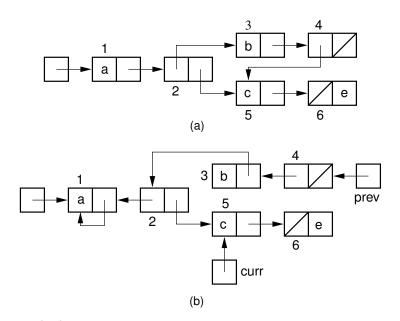
**Figure 12.18** Example of the Deutsch-Schorr-Waite garbage collection algorithm. (a) The initial multilist structure. (b) The multilist structure of (a) at the instant when link node 5 is being processed by the garbage collection algorithm. A chain of pointers stretching from variable **prev** to the head node of the structure has been (temporarily) created by the garbage collection algorithm.
