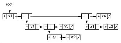
**Figure 12.4** Linked representation for the pure list of Figure 12.1. The first field in each link node stores a tag bit. If the tag bit stores "+," then the data field stores an atom. If the tag bit stores "-," then the data field stores a pointer to a sublist.
