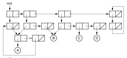
**Figure 12.5** LISP-like linked representation for the cyclic multilist of Figure 12.3. Each link node stores two pointers. A pointer either points to an atom, or to another link node. Link nodes are represented by two boxes, and atoms by circles.
