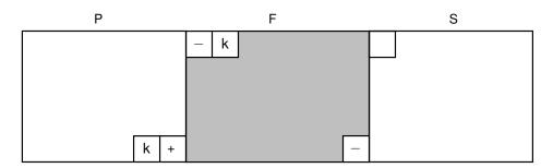
**Figure 12.13** Adding block F to the freelist. The word immediately preceding the start of F in the memory pool stores the tag bit of the preceding block P. If P is free, merge F into P. We find the end of F by using F's size field. The word following the end of F is the tag field for block S. If S is free, merge it into F.
